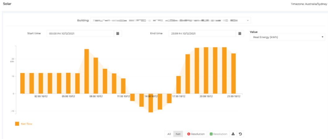
The solar tab showing the net energy flow (import/export) over a one day period
