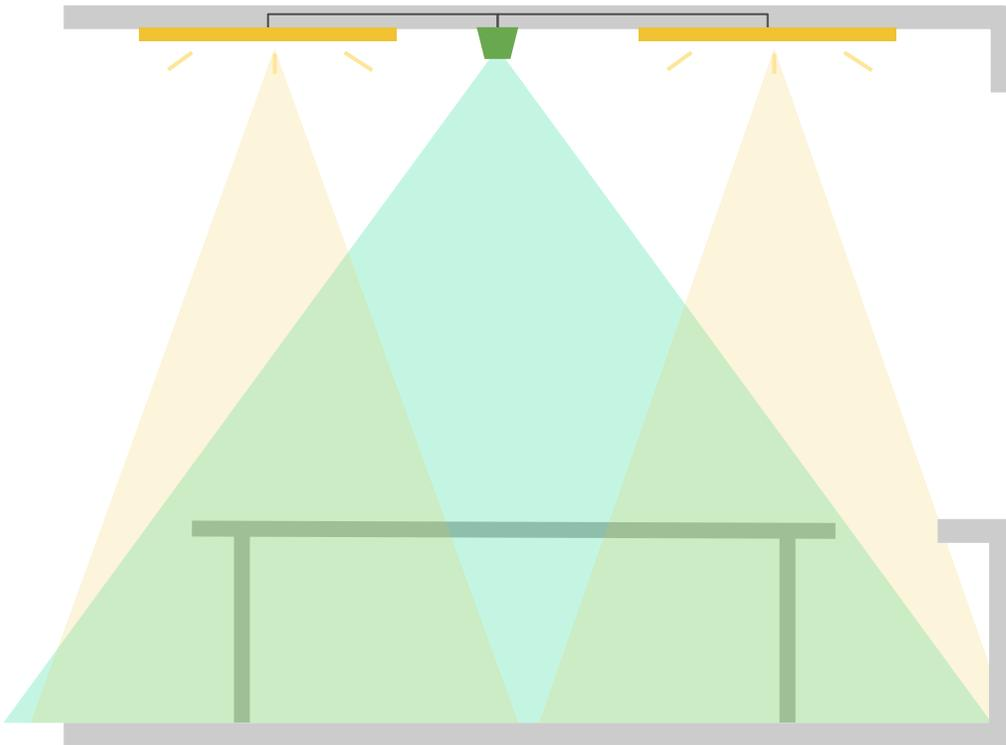
Sensor is controlling the light contributing to the field of view AND the controlled light contribute only to the sensor field of view.
