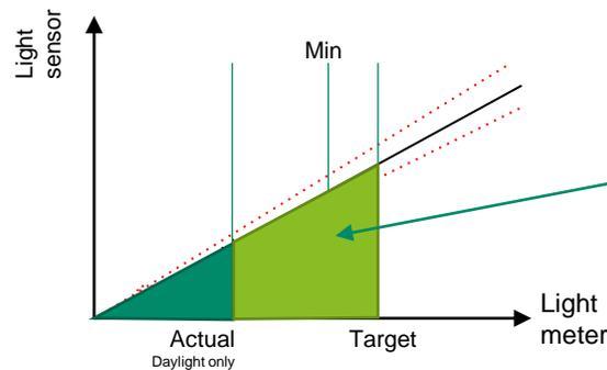
Use advanced setting in Calibration to increase level of lights to meet min level or target
