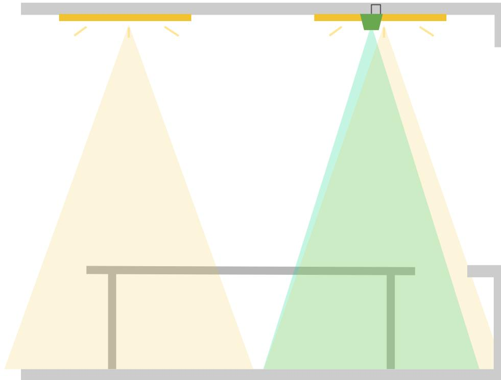
Sensor is controlling the light contributing to the field of view AND the controlled lights contribute only to the sensor field of view. The sensor is not affected by the light coming outside of the desired field of view.
