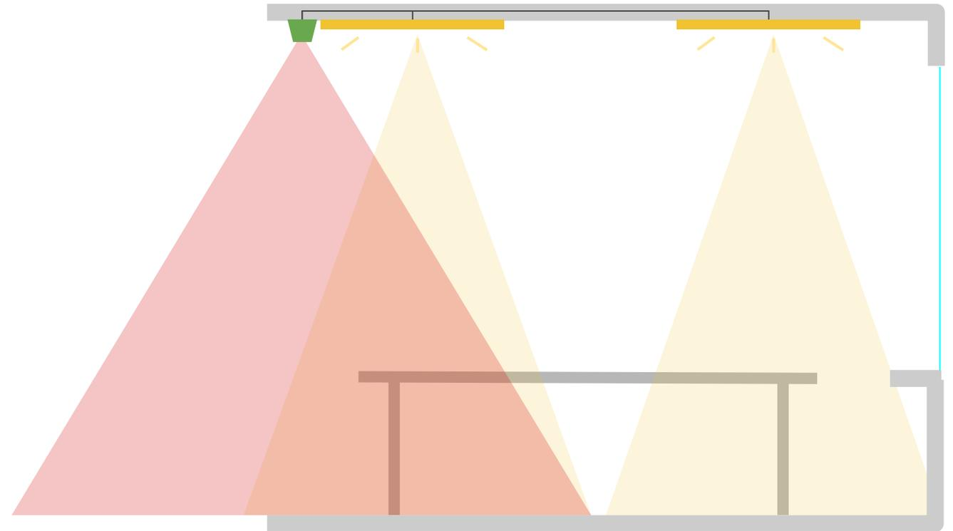
Sensor is not controlling the light contributing to the field of view OR the controlled light does not contribute to the sensor field of view.
