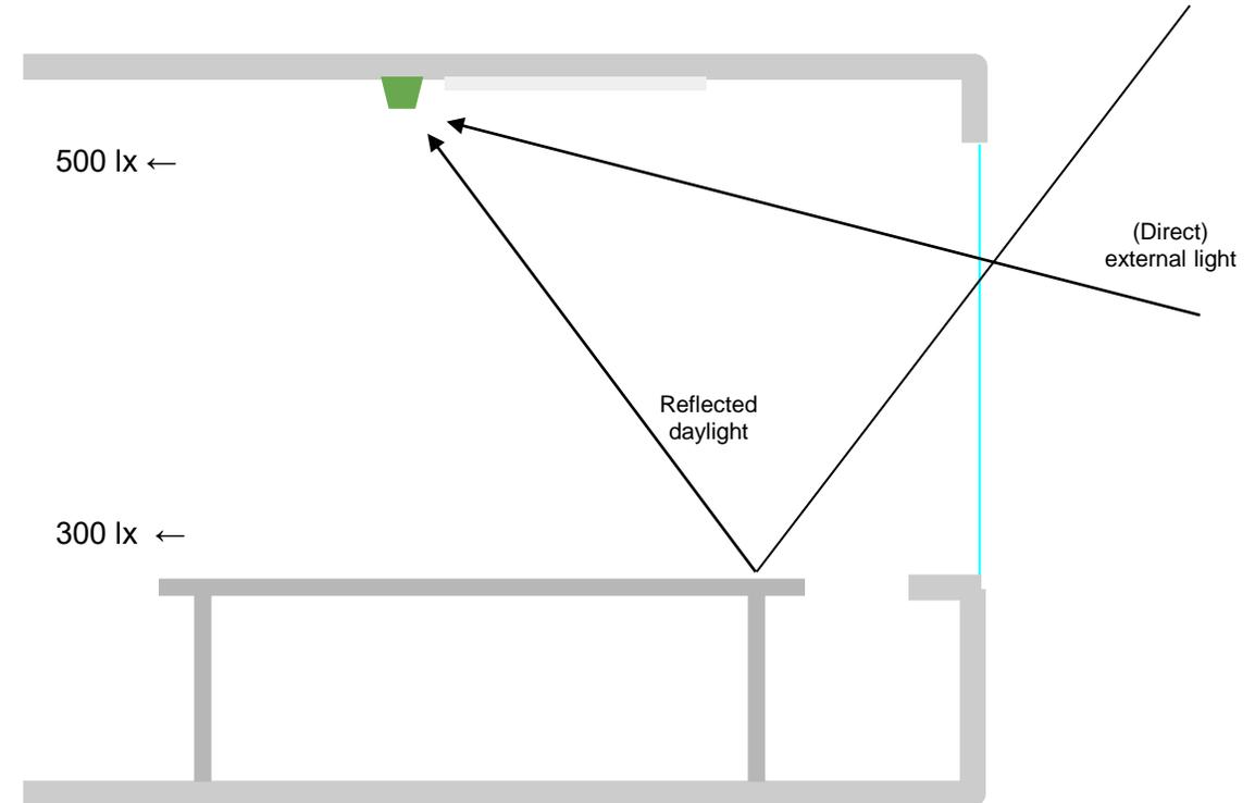
**During the day** external light is affecting the sensor and provides oversaturation error to the light level measured by the sensor which is higher than the light available on the surface (increased with the influence of the external light) which **leads to space being under-lit**.
