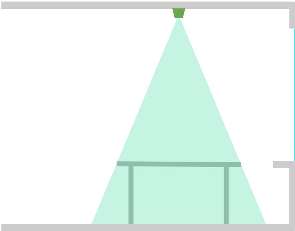
Sensor is installed above the surface where the light level needs to be maintained and is not affected by the external light.
