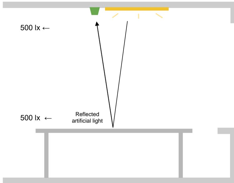
Sensor is **calibrated** with artificial light only **during the night**.
