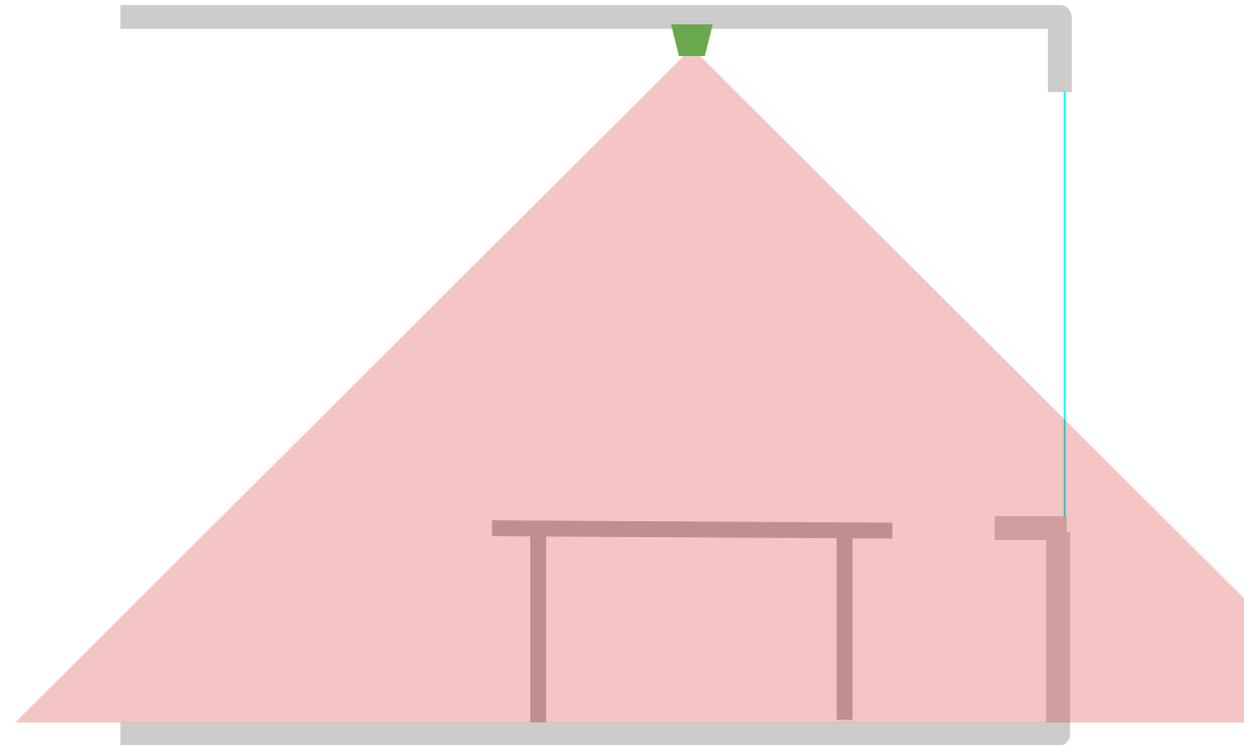
Sensor is installed above the surface where the light level needs to be maintained BUT due to the wide angle of detection the field of view is affected by the direct light coming out of the space (e.g. light reflected from a car rooftops)
