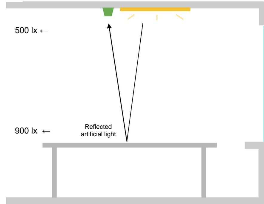
**During the night** external light is not affecting the sensor so the level of light measured by the sensor is lower (decreased by the lack of influence of the external light) than the light available on the surface which leads to **space being over-lit**.
