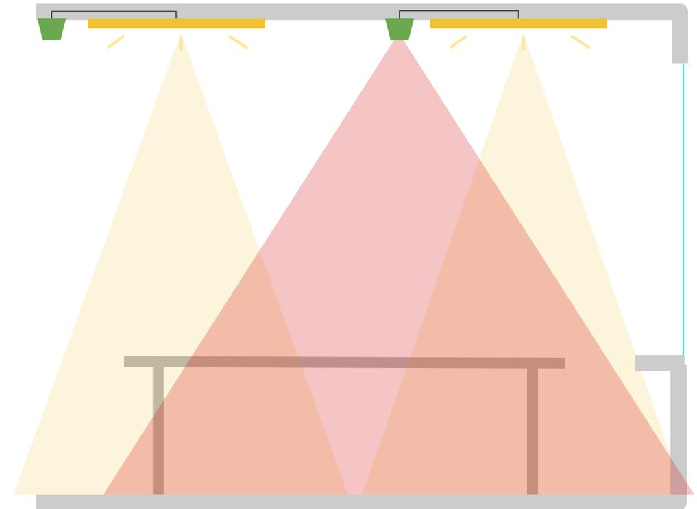
Sensor is not controlling all the lights contributing to the field of view. The sensor is affected by the light coming outside of the desired field of view, e.g. light controlled by other sensors.
