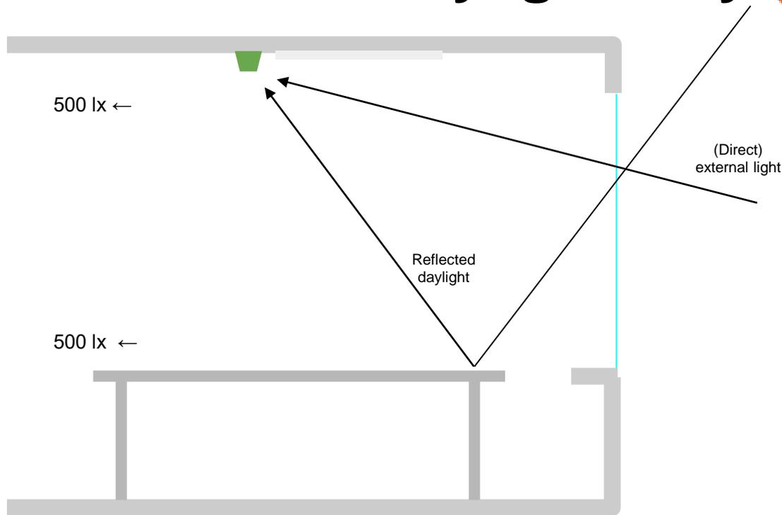
**Sensor is calibrated during the day** with daylight only including (direct) external light coming out of the field of view and sensor is calibrated with the error.
